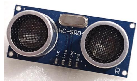
Picture 1 – HC-SR04 ultrasonic sensor has a speaker (T) and receiver (R) on the same board and uses only 4 pins.
