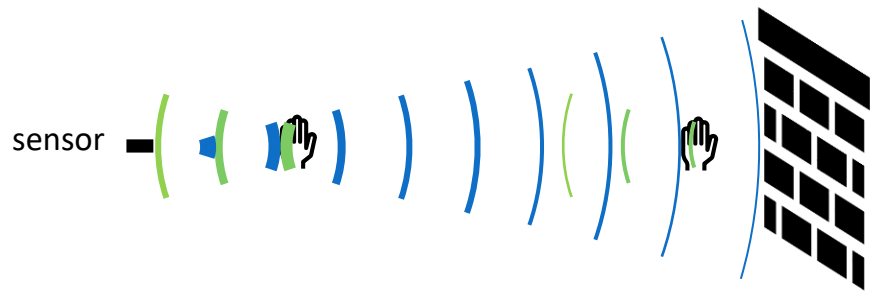
Picture 2 – on the left the small black square marks the position of the sensor. As the ultrasound spreads from the sensor its intensity gets smaller. A hand sized object can reflect most of the wave when it is close, but when it is further away it is just not large enough and will not be detected. At maximal distance you may need a wall sized object to reflect enough of the sound back.
