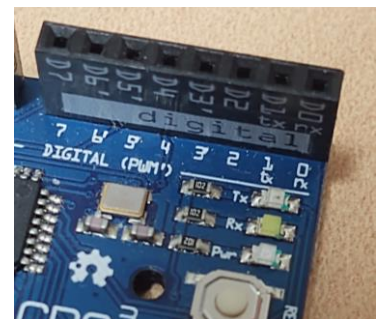
Picture 1 – take note of RX and TX markings next to the pins, and the LEDs
